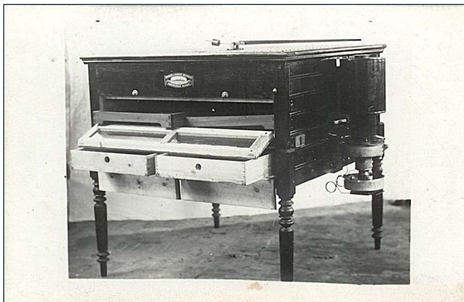
Advertising picture postcard of an incubator for hatching chickens, with regulated temperature system on the right.
